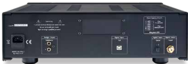
ABOVE: Back to basics with single-ended RCA outputs, a coaxial digital output and digital inputs for optical (to 96kHz, DSD64 DoP) and USB-B (384kHz, DSD128) sources
