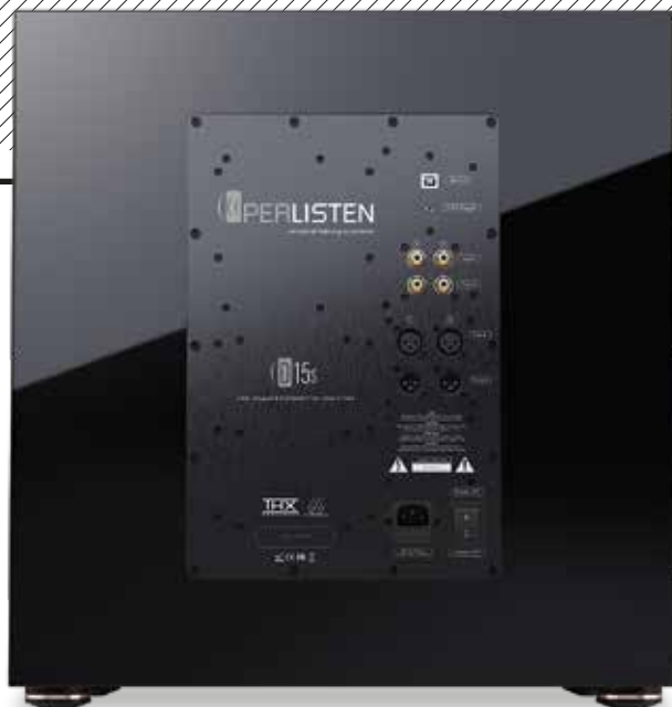
LEFT: Rear panel offers stereo/LFE inputs, and 'pass-through' outputs, on single-ended and XLR, plus a 3-12V trigger and USB-B (service) port. Full user controls are found on Perlisten's app
