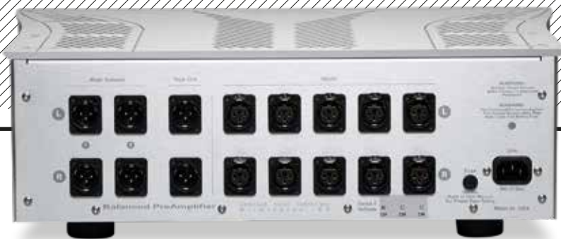
ABOVE: Five balanced inputs, one line/tape monitor output and two preamplifier outputs – all on XLR connections. Sources and systems with single-ended/RCA sockets will need adapters for use with BAT's VK-90
