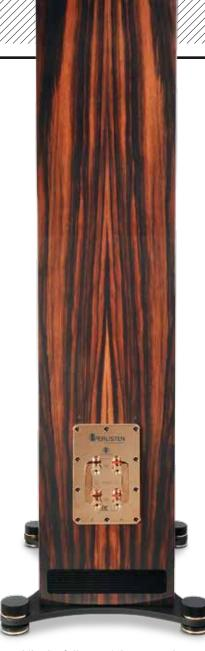
LEFT: The S5t's three-way (1.2kHz/ 4kHz) crossover is split between the bass/mid and DPC array drivers enabling bi-amping/bi-wiring if the gold-plated links (seen here) are removed. Side and rear vents come into play if the S5t is configured in reflex mode
