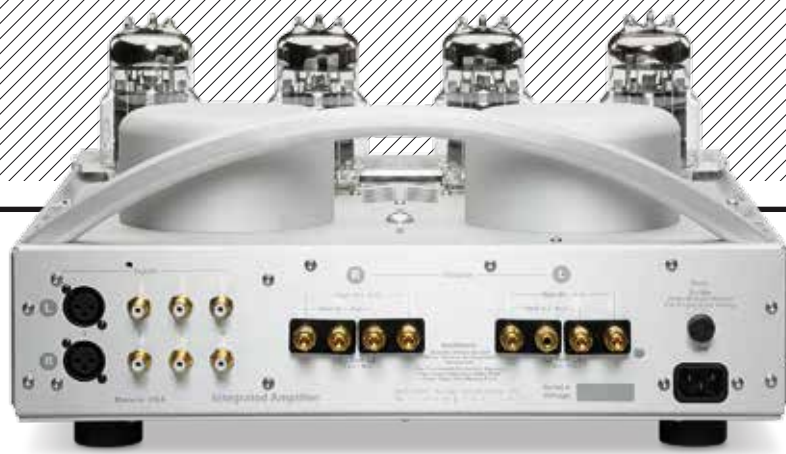
ABOVE: One balanced (XLR) and three single-ended (RCA) inputs are joined by rows of 4mm speaker terminals configured for 'High', 'Med' and 'Low' speaker impedances
