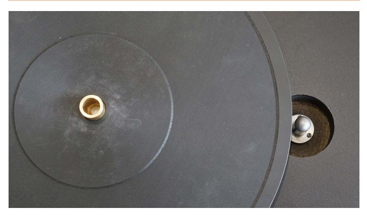
The underside of the StudioDeck's Delrin platter (left) showing its bronze sleeve with teflon thrust plate bearing that rotates around the fixed large steel pin in the plinth (right)
