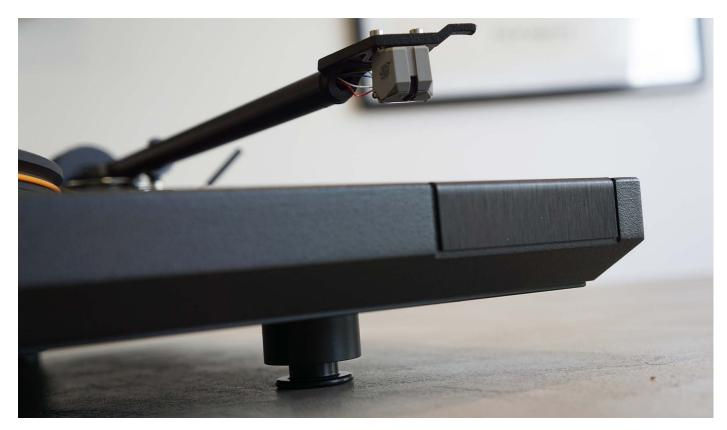
Four sprung feet help to isolate the deck from external vibrations. The rear feet have thicker pads, accounting for the extra mass at the deck's rear
