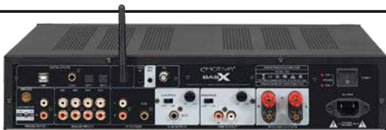
ABOVE: Four line, MM/MC and HT/sub ins sit alongside filtered low-pass (sub) and high-pass line outs, all on RCAs. Two optical, one coax and USB-B digital ins (192kHz/24-bit) are joined by FM and BT antenna(s). Speaker outs are via 4mm binding posts
