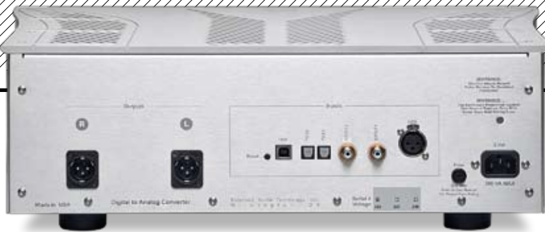
ABOVE: Six digital inputs are fitted including AES/EBU (XLR), S/PDIF (two on RCA and two optical) and USB-B for computer connection. Fixed analogue outputs are offered on balanced (XLR) connections only
