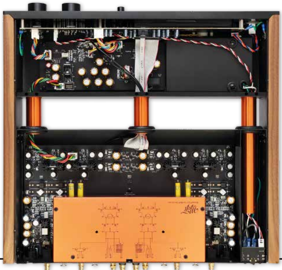
RIGHT: The two chassis enclosure, with PSU and logic [top] separated from current/voltage mode inputs, passive RIAA and balanced outputs [bottom], includes 'communication' via three copper-coloured tubes. Inputs are screened under a metal can that carries a basic schematic
