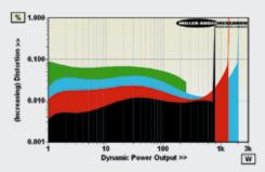
ABOVE: Dynamic power output versus distortion into 80hm (black trace), 40hm (red), 20hm (blue) and 10hm (green) speaker loads. Max. current is 32.1A
