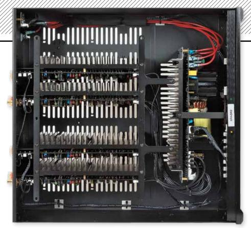
ABOVE: Inside the XPA-DR2's chassis a 3kW switch-mode PSU [far right] services a pair of Emotiva's Class AB/H 'Differential Reference' modules [centre left]. This chassis can accommodate up to three amplifier modules, becoming the £2150 XPA-DR3, with all three channels running off the same PSU
