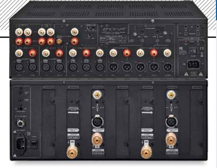
ABOVE: The preamp [top] offers six line inputs (four on RCA, two balanced on XLR), one MM/MC phono input, a processor/tape loop, L/R/Sub HT inputs and outputs, plus main outs (RCA and XLR). The power amp [below] has single-ended (RCA) and balanced (XLR) inputs with fully floating (ungrounded) speaker outputs
