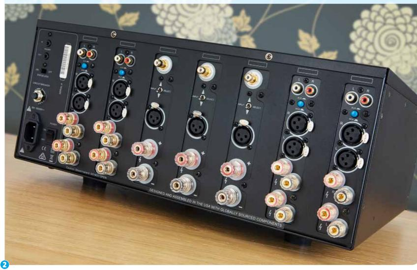
Such a configuration makes sense as the front three channels are critical for music, as well as creating a solid LCR soundstage with clear dialogue. The remaining eight channels handle surround and overhead or height speakers. Each channel of amplification employs a fully analogue Class AB output stage originally developed for Emotiva's first- and second-generation XPA devices.
