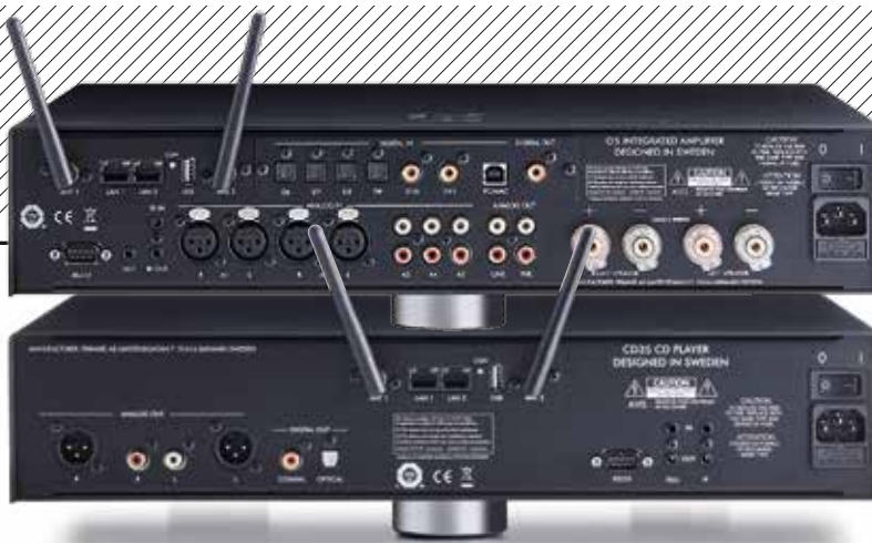
ABOVE: The amp [top] and CD player [bottom] include USB-A and Ethernet/Wi-Fi for Airplay, Bluetooth, Chromecast and Spotify. The I35 has four opt, two coax and USB-B digital ins alongside five line ins (two balanced on XLRs), pre out/line out and 4mm speaker terminals. CD35 includes balanced (XLR) line outs with coax/opt digital outs
