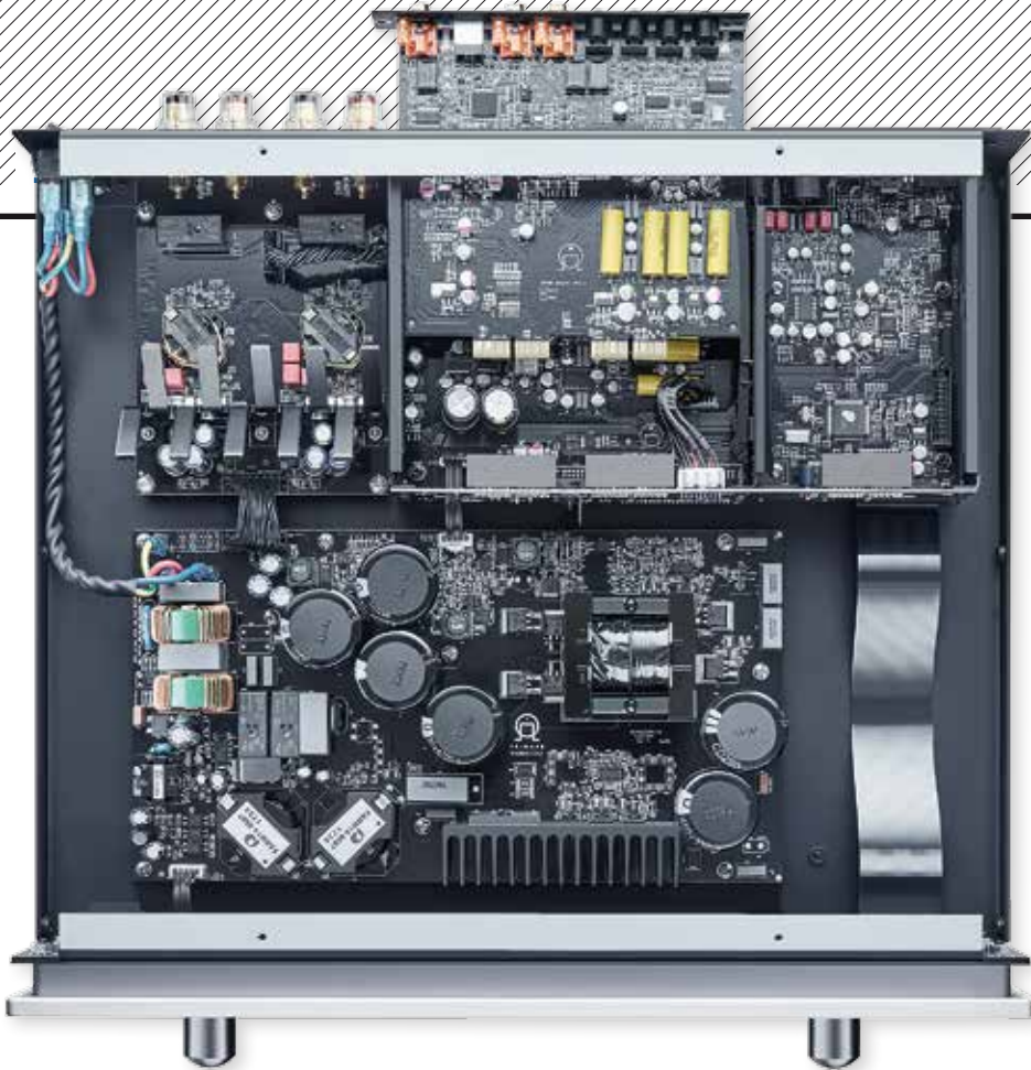
ABOVE: The I35 employs a very sophisticated switchmode PSU [main PCB] with differential PFC (Power Factor Correction), extensive filtering and separate regulation for the UFPD 2 Class D amp [top left]. Optional digital board [top] and network/Prisma board [top right] are individually screened
