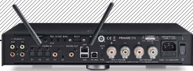
ABOVE: Wired/wireless network streaming (Bluetooth, Airplay, Spotify, Chromecast) is offered alongside a coaxial, 3.55mm mini-plug and three optical S/PDIF ins, a USB-B port and one analogue line in/out. Speakers are served by 4mm binding posts
