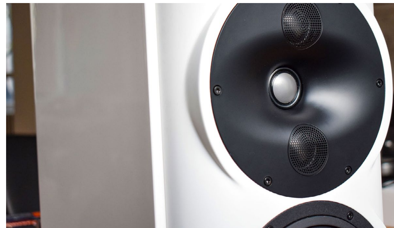
The tweeter array of the Perlisten Audio S5M is a true work of art. The beryllium dome tweeter in the center is supported by a horn-like waveguide. The supporting tweeters physically sit further forward.
