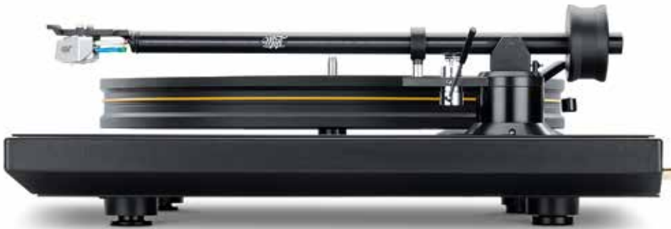
ABOVE: The heavyweight 10in Ultra tonearm has an aluminium main tube and friction-locked counterweight. It has provision to adjust azimuth at the headshell and VTA at the arm base
