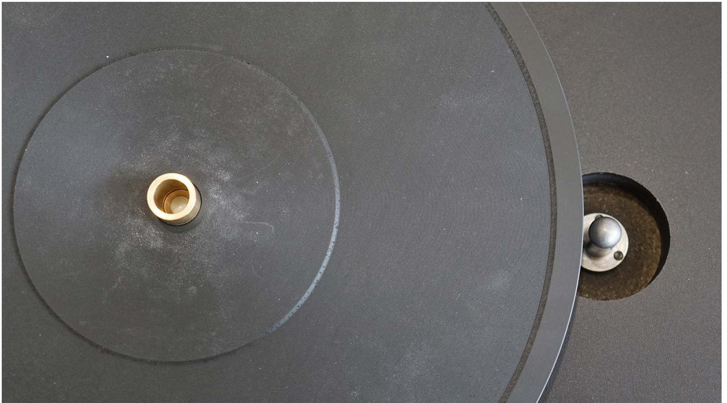
*The underside of the StudioDeck's Delrin platter (left) showing its bronze sleeve with teflon thrust plate bearing that rotates around the fixed large steel pin in the plinth (right)*
