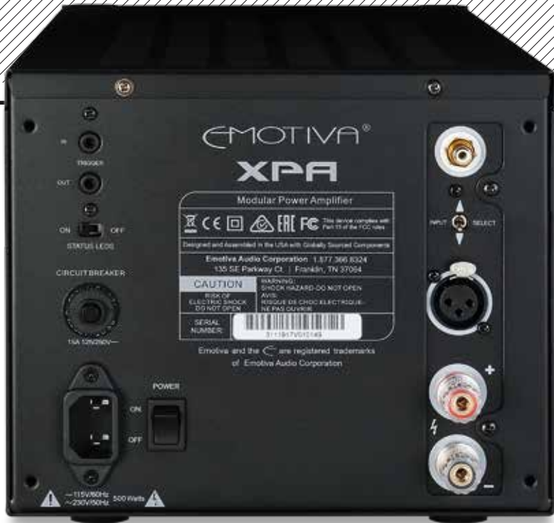
ABOVE: Single-ended (RCA) and balanced (XLR) inputs are switched via a toggle while outputs are limited to a single set of 4mm speaker terminals. The blue illumination can be defeated here while trigger ports assist with home/system automation
