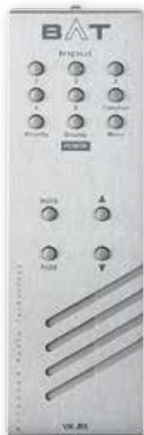
LEFT: BAT’s all-alloy VK-R5 remote provides access to input selection, volume, mute and limited display and menu items
